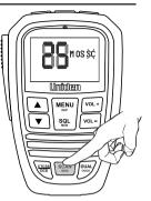
Press [SCAN] and scanning of the current memory group will start. SC flashes during scan.
