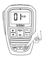
If scanning stops on a channel which is not a Priority Channel, the UHF CB Radio will continue monitoring the Priority Channel for activity while listening to the active one.
