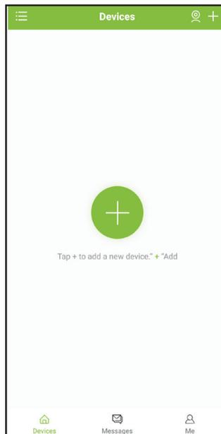
6. Please ensure the camera is powered on and is within the range of the router. Tap “Next” to continue. If the indicator light on the camera is not flashing slowly, press and hold the reset button with the reset pin for 5 seconds to reset the camera and set it up within 2 minutes. When the camera is flashing slowly, the camera is ready to set up tap “Next” to continue.
